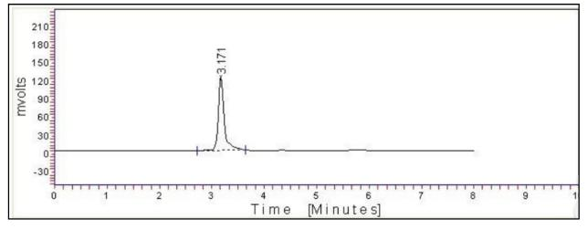
Fig. 1. Standard Chromatogram of Gallic acid.
